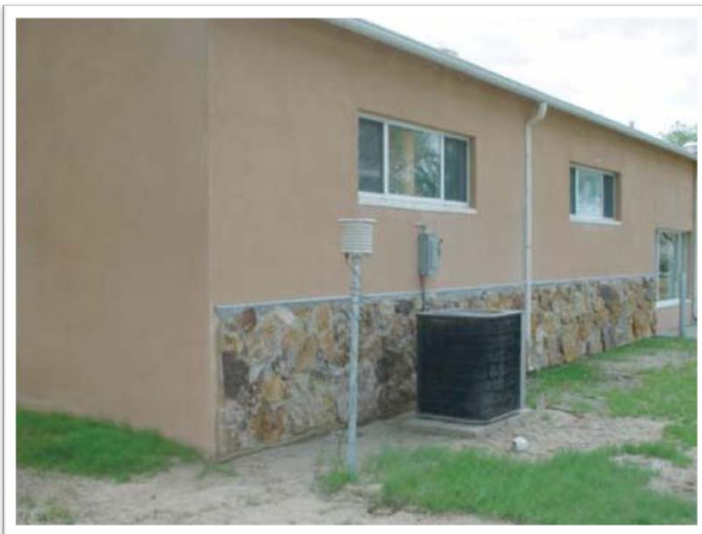
Max/Min temperature sensor near John Martin Reservoir, CO (Davey, 2005)
